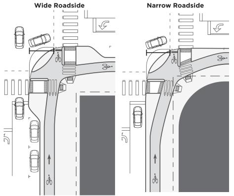
Wide roadside environment offer ample room to position safety islands and set back the bicycle and pedestrian crossings within the right-of-way limits. Narrow roadside environments with minimum dimension sidewalks and separated bike lanes offer little extra space for maneuvering or queuing within the right-of-way. Acquisition of additional right-ofway at corners may be necessary.
