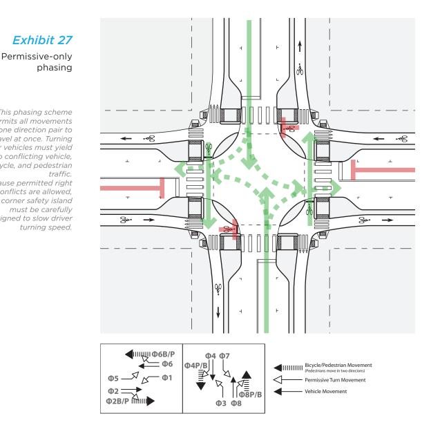
This phasing scheme permits all movements in one direction pair to travel at once. Turning motor vehicles must yield to conflicting vehicle, bicycle, and pedestrian traffic. Because permitted right turn conflicts are allowed, the corner safety island must be carefully designed to slow driver turning speed.
