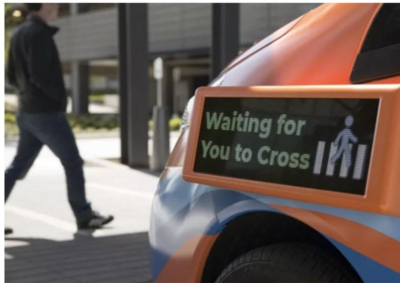
A screen mounted to the outside of an AV to describe the vehicle's intention to pedestrians. This method was proposed by drive.ai, a self-driving car company in operation in the US (Image: drive.ai).
